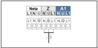
Fig.: Connection, heating circuit pump
