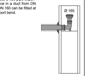
To check the balanced flue, undo and remove the cover of the inspection piece (3).
