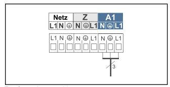
Fig.: Connecting output A1
