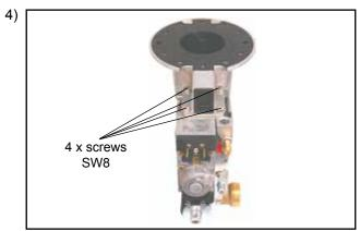
Undo the gas combination valve from the mixing chamber for gas/air (four SW8 screws).
