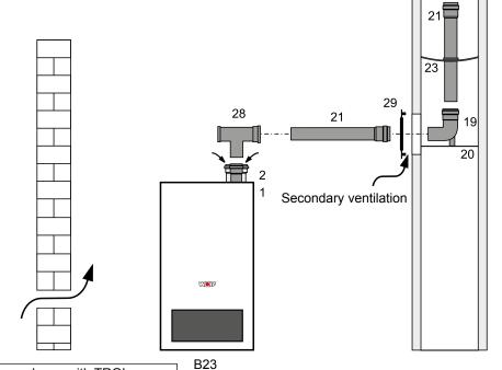
Ventilation air in **open** flue operation in accordance with TRGI:
