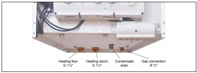
Fig.: Connections with heating circuit connection set (accessory)
