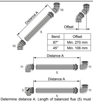
always be approx. 100 mm longer than distance A. Always trim the flue on the smooth side, never on the female connection side.
