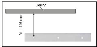
Fig.: Drill holes for suspension bracket
