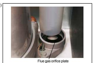
Place the flue gas orifice plate Ø 53 mm into the condensate pan and insert the flue pipe again.
