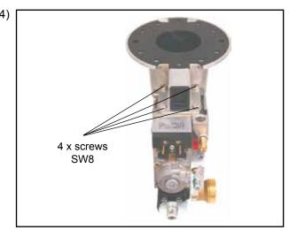
Undo the gas combination valve from the mixing chamber for gas/air (four SW8 screws).
