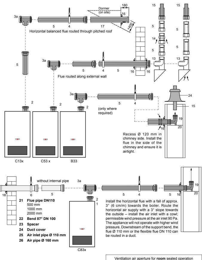
Ventilation air aperture for **room** sealed operation according to TRGI 150 cm<sup>2</sup> or 2 x 75 cm<sup>2</sup>.
