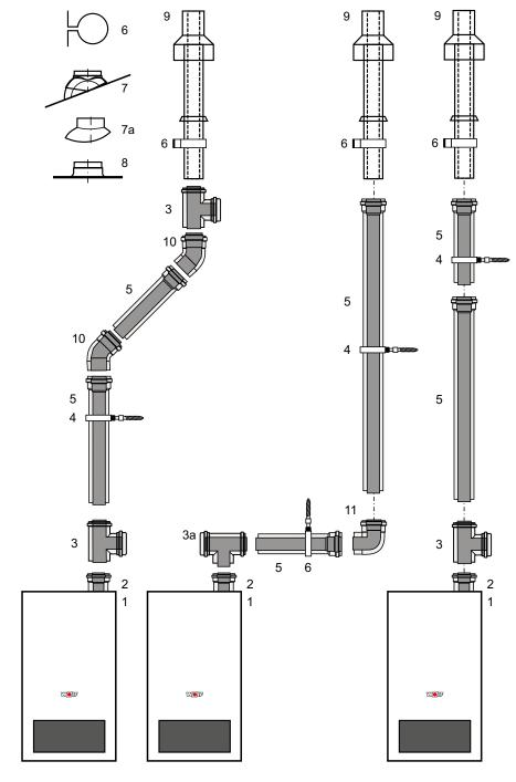
Type C33x: Gas condensing boiler with combustion air and flue gas routed vertically via the roof.
