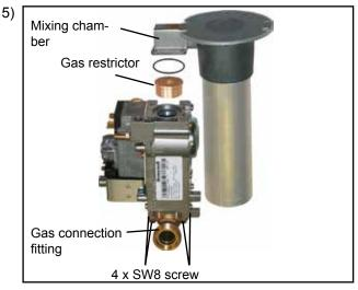
Remove the four SW8 screws at the gas connection fitting and remove the fitting from the gas combination valve. Remove the gas combination valve and gas restrictor. Place the protective labels at the valve inlet and valve outlet of the new gas combination valve at the apertures of the removed valve.
