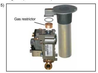
Remove integral gas restrictor and replace with the gas restrictor for the new gas type (in accordance with the table on page 25).
