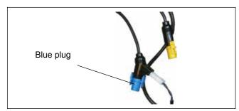
Fig.: Blue plug for cylinder sensor connection
