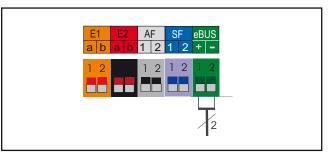
Fig.: Connecting digital Wolf control accessories (eBUS interface)
