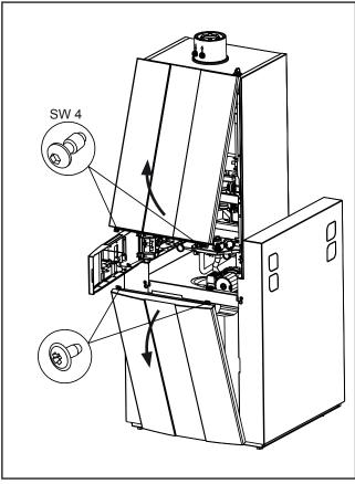
Fig.: Dismantling the stratification cylinder front casing
