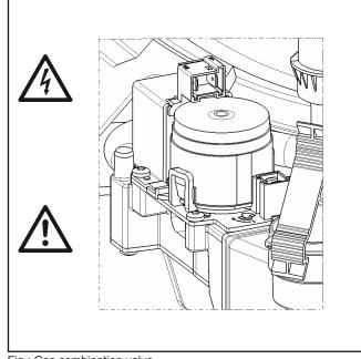
Fig.: Gas combination valve Danger through live electrical components Escaping gas may cause poisoning or an explosion
