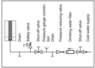
Fig.: Cold water connection to DIN 1988
