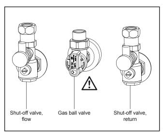
Fig.: Gas connection: Risk of poisoning or explosion in the event of gas escaping
