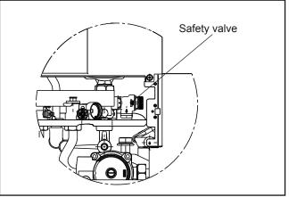
Fig.: Heating circuit safety valve (CGS-2L shown)
