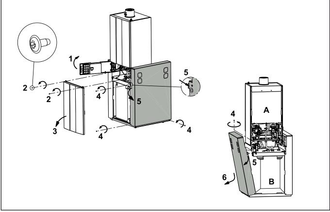
Fig.: Dismantling the CGS-2L/R side cylinder casing
