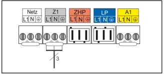
Fig.: Connecting output Z1
