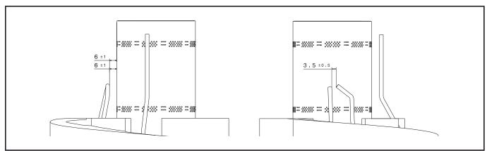
Fig.: Ignition electrode gap
