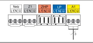
Fig.: Connecting output A1
