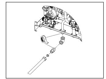
Fig.: Gas connection installation
