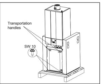
Fig.: Front transportation handles/locking screws
