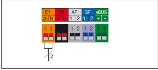
Fig.: Connecting input E1
