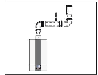
Fig.: Example: Balanced flue
