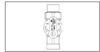
Fig.: Gas ball valve, straight (accessory)
