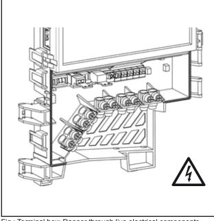
Fig.: Terminal box: Danger through live electrical components
