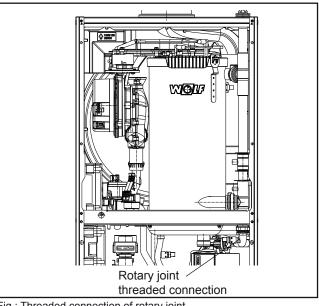
Fig.: Threaded connection of rotary joint
