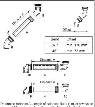
approx. 100 mm longer than distance A. Always trim the flue on the smooth side, never on the female connection side. Chamfer the flue with a file after trimming.
