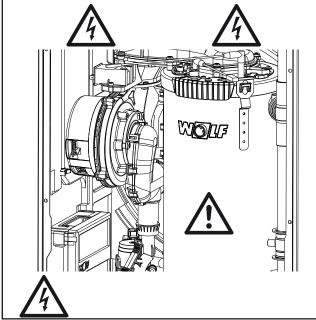
Fig.: Ignition transformer, high voltage ignition electrode, combustion chamber
