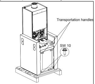
Fig.: Back transportation handles/locking screws
