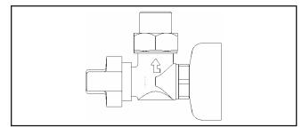
Fig.: Gas ball valve, angled (accessory)
