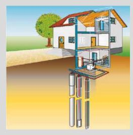
System scheme - geothermal probe
