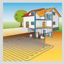
System scheme - geothermal collector
