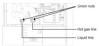
Fig.: Connecting the refrigerant lines to the indoor module
