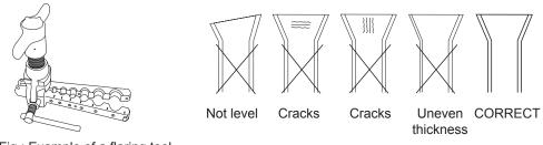
Fig.: Example of a flaring tool
