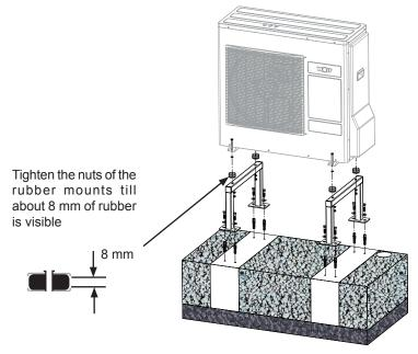
Cast, level plinth of concrete with gravel base providing sufficient frost protection, cut-out for cable/line entry, see foundation diagram
