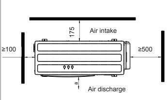
Fig.: Plan view of outdoor module BWL-1S(B)-05/07
