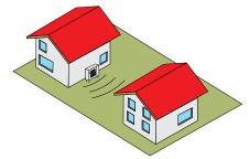
Q = 8: Heat pump or air intake/discharge (indoor installation) on a house wall with recessed corner in exterior wall
