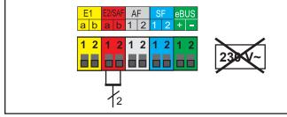
Figure: Input E2/SAF connection
