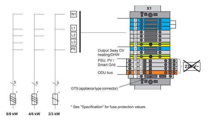
On the BWL-1S with integral 3-phase electric heater, the heater connection can be either single phase, 2-phase or 3-phase. Depending on demand, the control unit activates the electric heater via a contactor.
