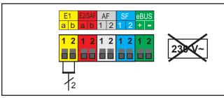
Figure: Input E1 connection
