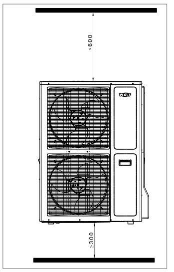
Fig.: Front view of outdoor module BWL-1S(B)-10/14/16
