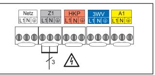
Figure: Output Z1 connection
