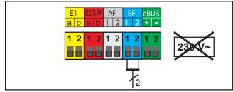
Figure: Cylinder sensor SF connection
