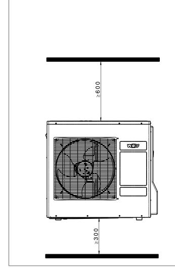
Fig.: Front view of outdoor module BWL-1S(B)-05/07
