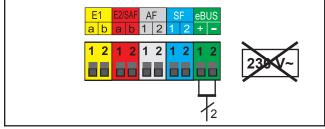
Figure: Connecting digital WOLF control accessories (eBUS interface)
