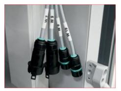
Prepared and encoded connectors for easy cabling.
