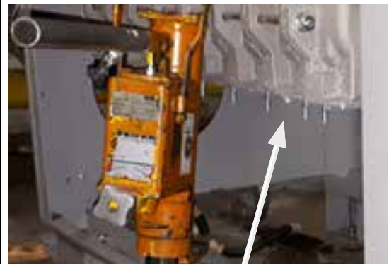
Jack beneath connecting rod
