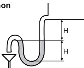
If the siphon is provided on site, calculate the height of the siphon in accordance with the sketch shown here.
