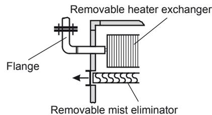
For the heat exchanger (with flange) it is recommended to use bends to make the connections. This configuration will ensure that the heat exchanger and the mist eliminator can be extracted to one side for subsequent cleaning.
