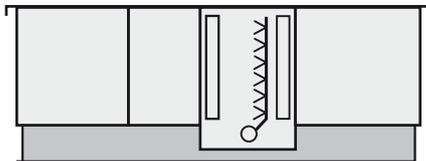
A base frame or plinth (height approx. 305 mm) is always required for KG or KGW appliances with scrubber, because the scrubber bottom lies lower than the underside of the remaining appliance. The required height of the base frame depends on the type of scrubber and is specified separately in the course of the design calculations.
