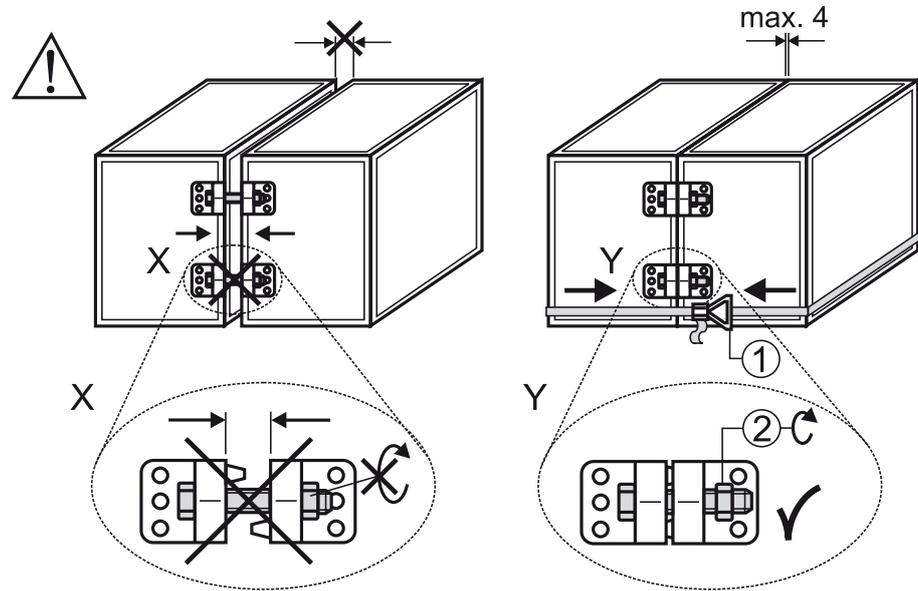
Tensioning straps may be used to make the assembly of the cube units easier. Position the appliance parts next to each other and close the gap between them with tensioning straps. Then bolt the components together by means of the connectors supplied.
