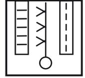
Heater section with frost protection frame
