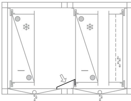
The tray bridge is already fitted in the factory if the functional components are delivered as a single transport unit.
