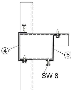
Connecting brackets, items 4 and 5, if air conditioning units are positioned next to each other (assembly on site)
