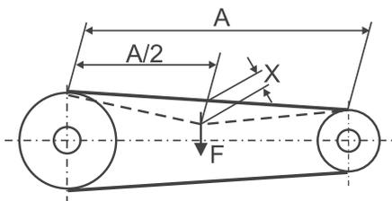
Always replace the complete set of vee-belts if one or several vee-belts require replacement on a multi-groove drive.
