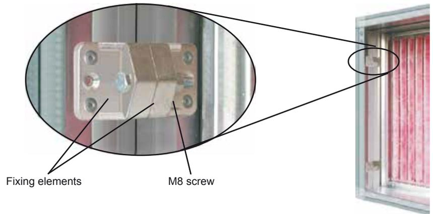
When tightening screws and nuts, always counterhold with a second open-ended spanner.
