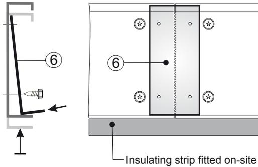
**Support bracket, item 6, in case of factory-fitted base frame, if different weights lead to an offset at cube joints (assembly on site)**
