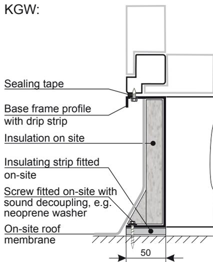
A base frame or plinth is required for air-handling units installed as weatherproof version to support the appliances and their components.
