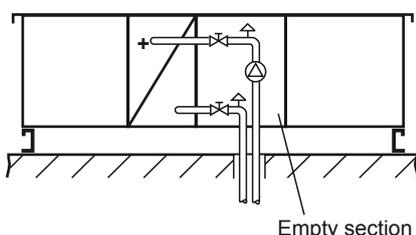
The weatherproof projection is not thermally insulated. **Consequently, the pipes and valves must be adequately insulated and, if necessary, heated on site. If an inverter is used for operation it is advisable to provide external ventilation in summer to prevent overheating (max. permissible temperature 45 °C). Provide suitable apertures through the removable base of the projection to accommodate the pipes.**
