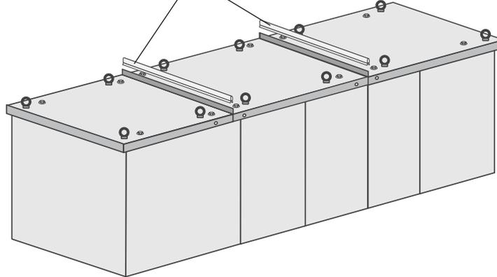
The roofs of the weatherproof appliances can be stepped on for assembly. Attention must be paid here to the area distribution of the load (boards).
