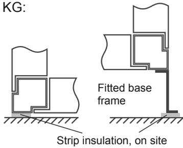
The base frame must be horizontal, and the foundation must be level and horizontal (check with browning rod).
