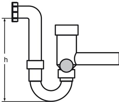
To permit reliable draining of condensate, it is important to connect a ball siphon to the condensate drain connector from the drain tray for the cooling coil / direct-expansion evaporator, plate-type heat exchanger and outside air intake tray of the KGW.
