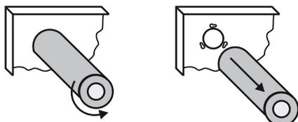
Replace the activated charcoal filters (cartridges) if they are saturated (expiry of the specified operating time).
