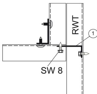
Connecting bracket, item 1, in case of connection to, for example, a rotary heat exchanger (assembly on site)
