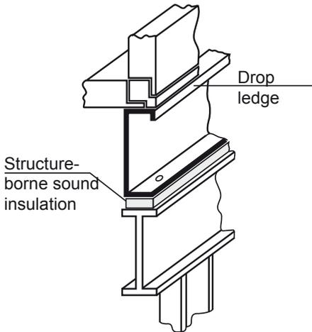
The WOLF base frame must be insulated and integrated into the roof sealing system on site.
